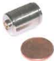
Small battery for smart artillery ammunition
