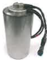
Thermal battery for fighter aircraft EPS
